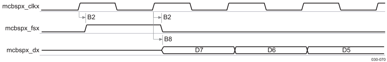
Figure 6-35. McBSP Rising Edge Transmit Timing in Master Mode
